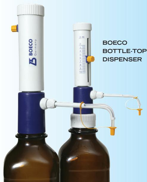
**BOECO Bottle-Top Dispenser, complete with 3 adapters, intake tube FEP, Discharge-tube (with safety thread) FEP, closure cap, without reservoir bottle.**
